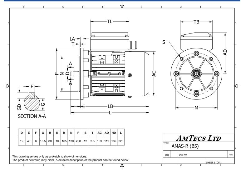
Specification IEC 60034-1 Manufacturer **AmTecs** Motor type AMAS-R 80G2 Rated power 1.1 kW S1 Duty Speed 2800 rpm Voltage 220V **50** Hz Frequency
