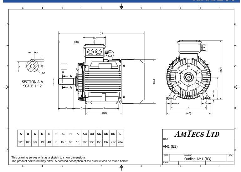
Specification IEC 60034-1 Efficiency class Manufacturer **AmTecs** Load data Motor type AM1-IE2 80G2 Efficiency Rated power **1.32** kW S1 Duty Power factor Speed 3450 rpm Voltage 277 / 480V **60** Hz Frequency Connection Delta / Star Full load current 4.1 A / 2.4 A Full load torque No-load current **IP55 Enclosure** F (temp. rise B) Insulation class Max. ambient temp 40 °C
