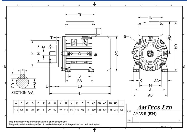
Specification IEC 60034-1 Manufacturer **AmTecs** Motor type AMAS-R 90L2 Rated power 2.2 kW S1 Duty Speed 2800 rpm Voltage 220V **50** Hz Frequency **Single Phase** Connection
