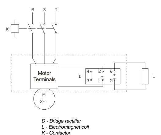
Connection diagram for slow braking.
