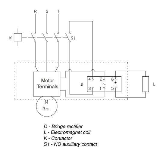
Connection diagram for fast braking.
