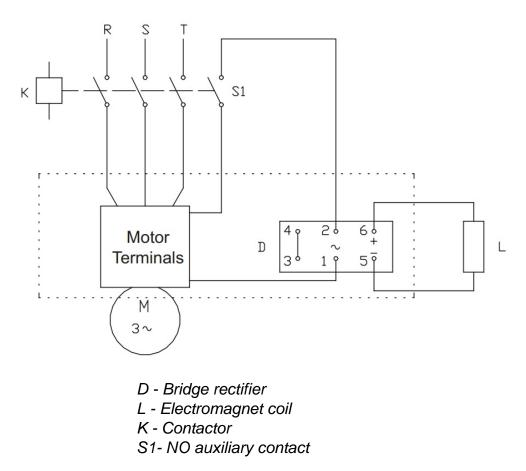
Connection diagram for medium braking.
