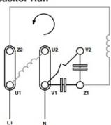
The below circuit shows a basic diagram of how to implement switching between both forward and reversing of a single phase motor.
