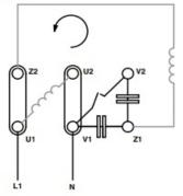
The below circuit shows a basic diagram of how to implement switching between both forward and reversing of a single phase motor.
