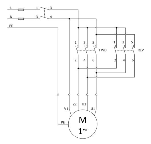
Note: It is important to not change the direction whilst the motor is running.
