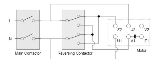
Note:It is important to not change the direction whilst the motor is running.
