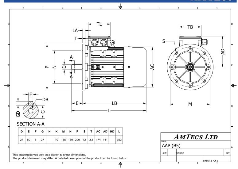
Specification IEC 60034-1 Manufacturer **AmTecs** Motor type AAP 90L2A Rated power 2.2 kW S1 Duty Speed 2875 rpm Voltage 220V / 400V **50** Hz Frequency Connection Delta / Star
