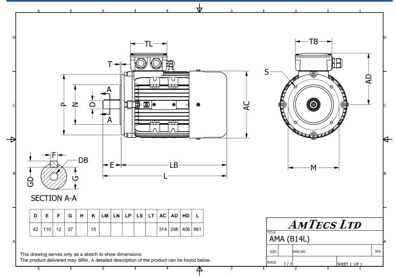
Specification IEC 60034-1 Manufacturer **AmTecs** Motor type **AMA-IE2 160L6** Rated power kW S1 Duty 11 Speed 970 rpm Voltage 400V / 690V **50** Hz Frequency Delta / Star Connection Full load current 22.9 A / 13.22 A No-load current **Enclosure IP55**
