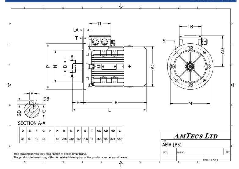
Specification IEC 60034-1 Efficiency class Manufacturer **AmTecs** Load data Motor type **AMA-IE2 132M6** Efficiency Rated power kW S1 Duty Power factor Speed 965 rpm Voltage 400V / 690V **50** Hz Frequency Connection Delta / Star Full load current 8.96 A / 5.17 A Full load torque No-load current **IP55 Enclosure** F (temp. rise B) Insulation class Max. ambient temp 40 °C
